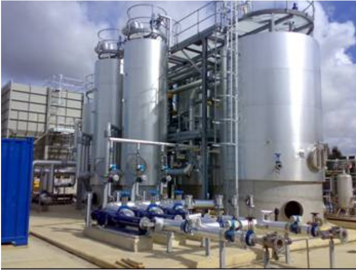
Figure 7: Typical Thermal Hydrolysis Plant for 20,000 dry tonnes sludge per year.
