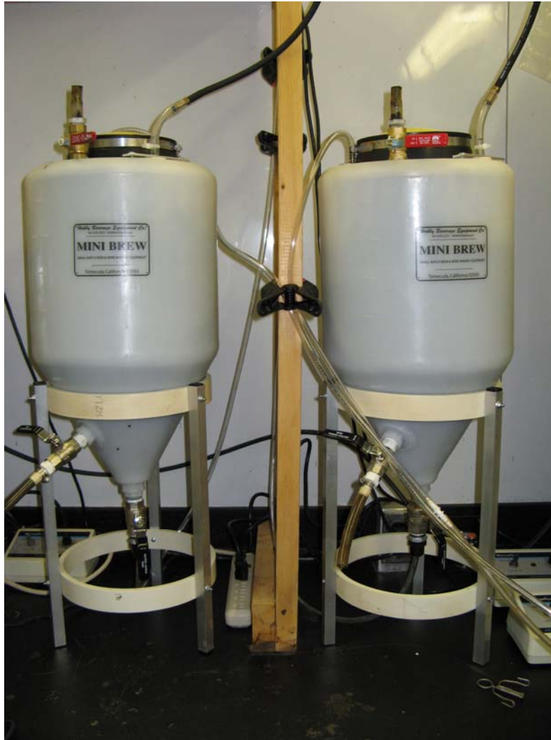
Figure 1. Bench scale mesophilic anaerobic digesters
